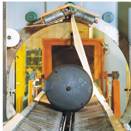
Cylinders are wrapped in foil before the CFC-free foam insulation is applied. This way, the materials can be easily segregated during disposal.
