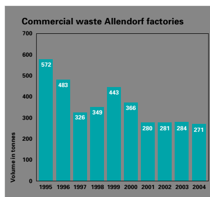
Reducing special waste by avoiding the use of bonding agents during the manufacture of composite duplex heating surfaces
